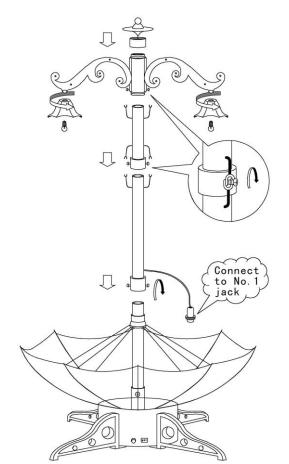
Assemble the street lamp components as shown on schematic and insert the plug at bottom into No. 1 jack in its base. Note: (a) To ensure normal functioning of the street lamp after power on, good contact of connection wires between each street lamp tube section shall be ensured. (b) Tighten each screw so that each lamp tube forms a strong base of the product.
